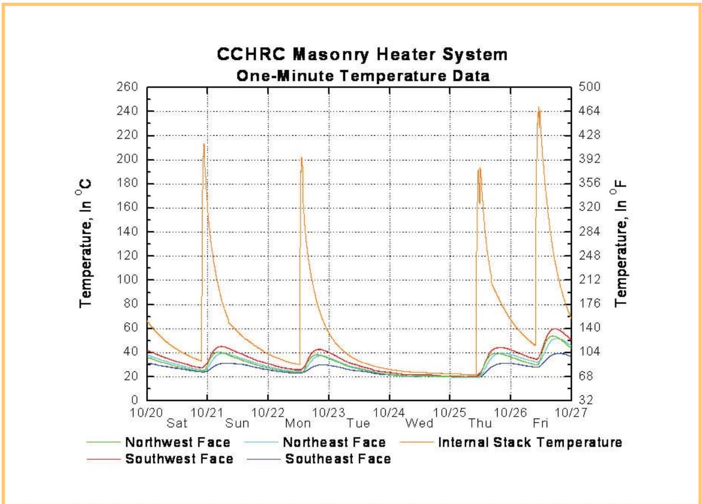
Figure 2. Temperature data for the masonry heater rock faces and stack. Measurements are taken every minute. Each increase in temperature is a unique burn. The cooling of the rock faces takes more than 24 hours to go back to ambient room temperature.
