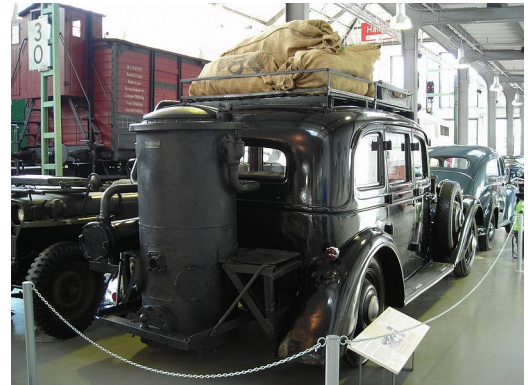
Figure 4: A 1941 car with a gas generator. Photo courtesy of Mattes and the Deutsches Museum Verkehrszentrum.
